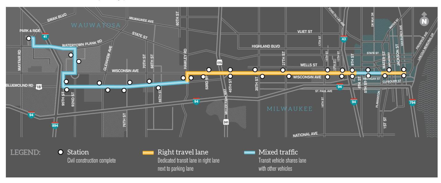
The dedicated bus lanes will occupy the right travel lane and will be designated using pavement markings and permanent signage. Access will be maintained to parallel parking and driveways. After yielding to buses, motorists will be permitted to enter the dedicated bus lane for right turns (both intersection and driveway) and parallel park in designated areas. Motorists are not allowed to travel in the dedicated bus lane.
